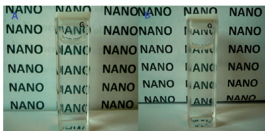
Figure 5. Photographic images of (A) oleate-capped (NaGdF 4 :3% Nd 3+ )/NaGdF 4 nanocrystals dispersed in hexane and (B) ligand-free (NaGdF 4 :3% Nd 3+ )/NaGdF 4 nanocrystals dispersed in water.
